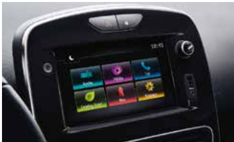
Main menu with 6 icons Radio, Multimedia, Telephone, Eco Driving, Navigation, System settings.
